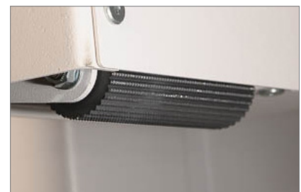
Improved PGO (Paper Grain Opening) Microcut spine roughening
