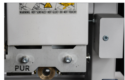
Closed PUR tank with glue applicator
