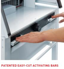
Blade and clamp can be activated independently via the two-step blade activating bars with separate trigger points for blade and clamp.
