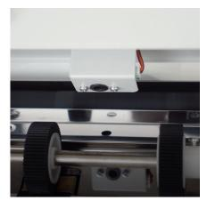
SENSOR FOR DOUBLE FEED DETECTION
