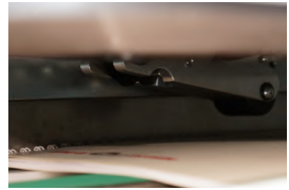
Wire-O® closing area with auto-centering of bound document
