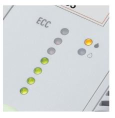
**ECC – ELECTRONIC CAPACITY CONTROL** This electronic feature indicates the used sheet capacity during shredding process to avoid paper jams.
