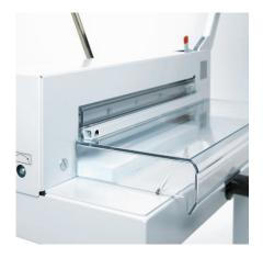
**TRANSPARENT SAFETY GUARD** A cut can only be executed, if the safety guard is closed and the safety catch for the blade
