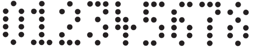
20 mm condensed, matrix 3 x 6, pin Ø 2.3 mm
